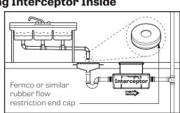
on the sink piping that discharges into the drain. See drawing above for guidance. For detailed guidance on indirect connections, go to: http://webtools.schierproducts.com/Technical\_Data/Indirect\_Connections.pdf
